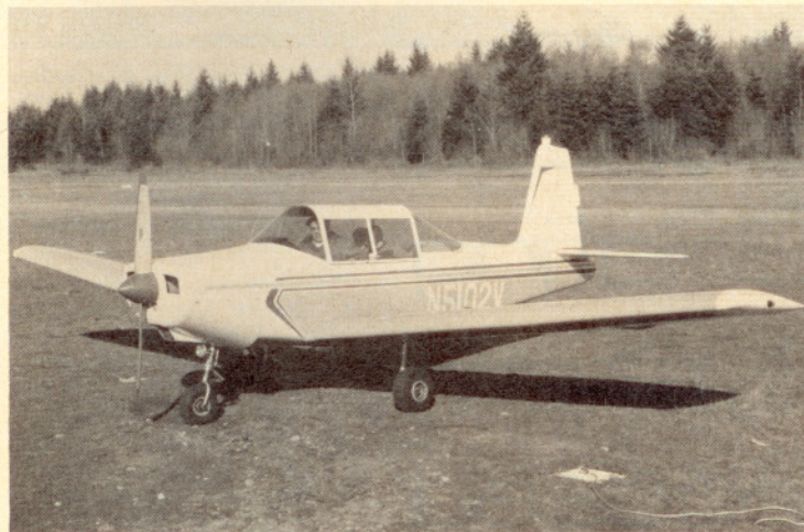
The original Morrisey Nifties had welded-steel-tube fuselages with fabric covering. This improved 2000 version had a metal wing and crimped-aluminum rudder and elevator. Plans for the 1000C with wood wing are now available to amateur builders.
